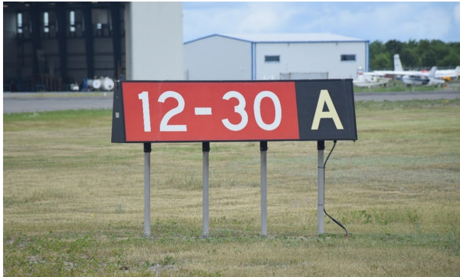
Figure 13 - Runway-Taxiway Intersection Mandatory Instruction and Location Sign
